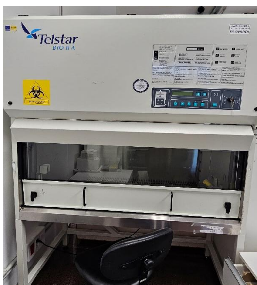
Figura 5. Cabina Telstar Bio II A.
